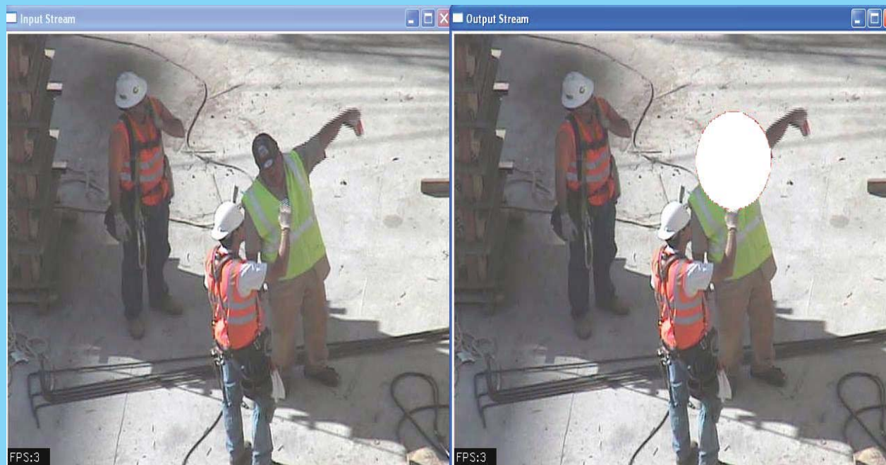
An example of the Respectful Camera system obscuring the face of the construction worker wearing a green vest.
